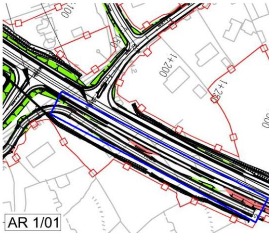
**Recommendation:** The Designer should assess the potential for headlight glare between opposing road users on the parallel access roads and the mainline. If it is found that headlight glare could be an issue appropriate mitigation measures should be introduced.
